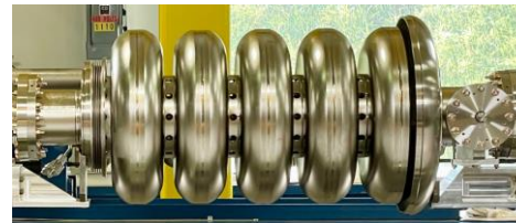
PIP-II LB650 SRF cavity
