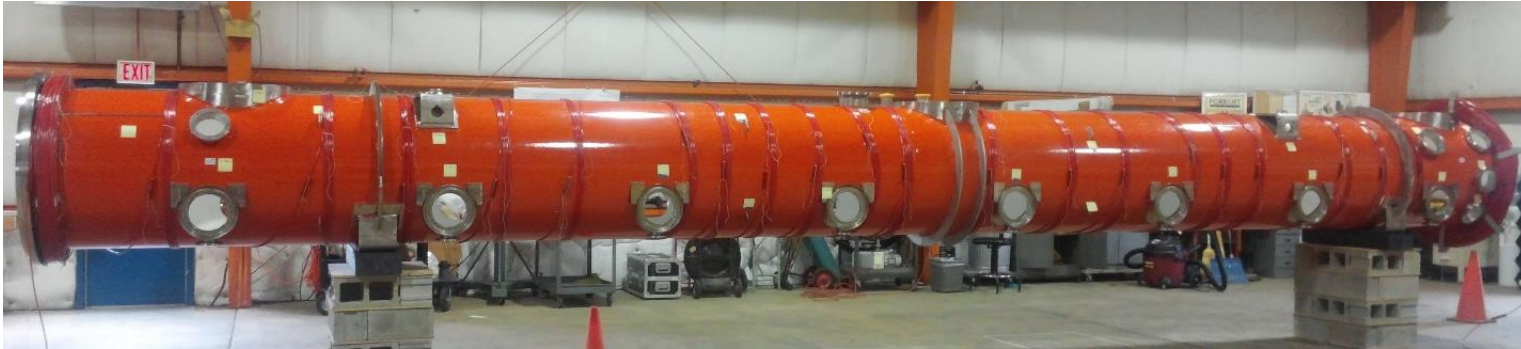
Helmholtz coils wound onto vessel directly
